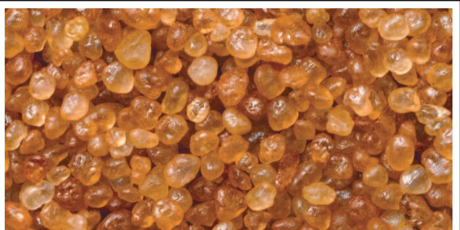
Momentive Specialty Chemicals Inc.'s OilPlus™ proppant is a resin-coated sand designed to increase oil flow through the proppant pack. Developed by its Oilfield Technology Group, the company describes OilPlus proppant as a curable, resin-coated sand with the bonding characteristics of a high-quality, resin-coated proppant.
